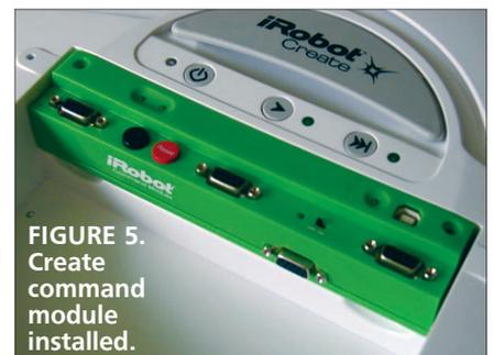
**FIGURE 5. Create command module installed.**
